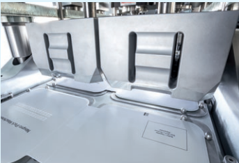
ULTRASONIC SEALING OF CARDBOARDS ONTO TRAYS
