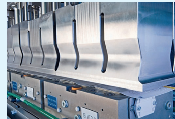
ULTRASONIC SEALING OF BACKING CARDS ONTO BLISTER
